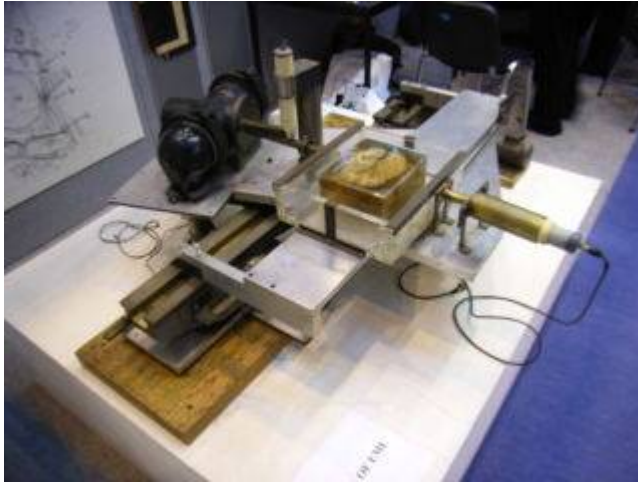
Figure 2. The very first CT scanner prototype. Invented by Hounsfield at EMI [12].
