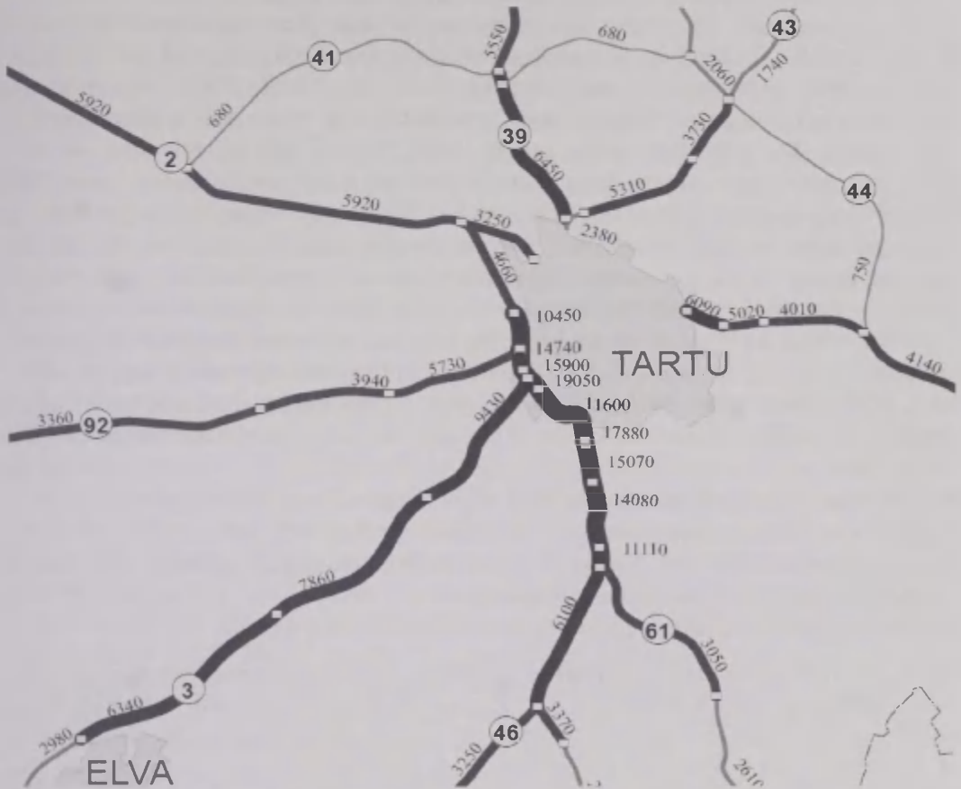
Fig. 7. Daily average traffic frequency on Tartu transit roads and bypasses (Roads Technocenter, 2007).
