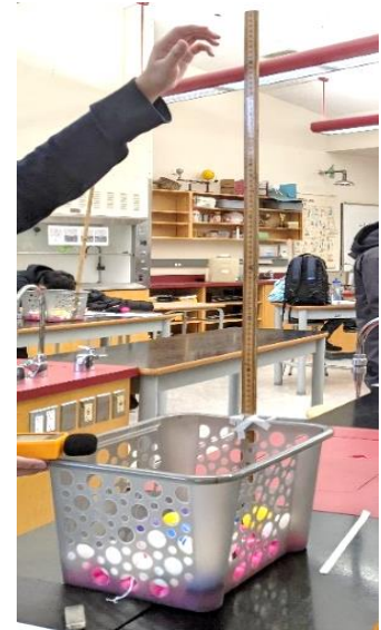
Figure 1 – A student sets up their apparatus, filling a basket with ping pong balls and securing a metre stick to the side of the basket to measure drop height
