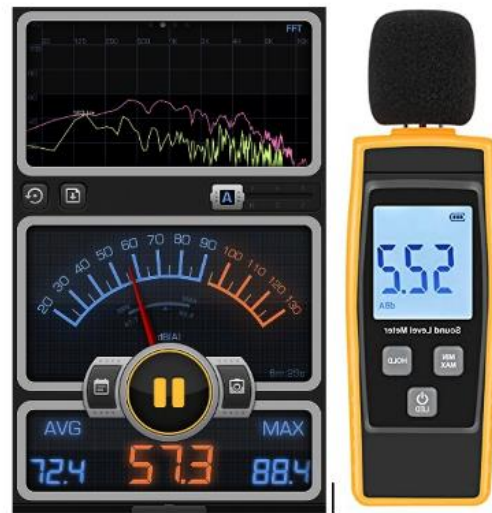
Figure 2 - A side-by-side comparison of the Decibel X interface (left) used on a smartphone, with that of the decibel meter (right)
