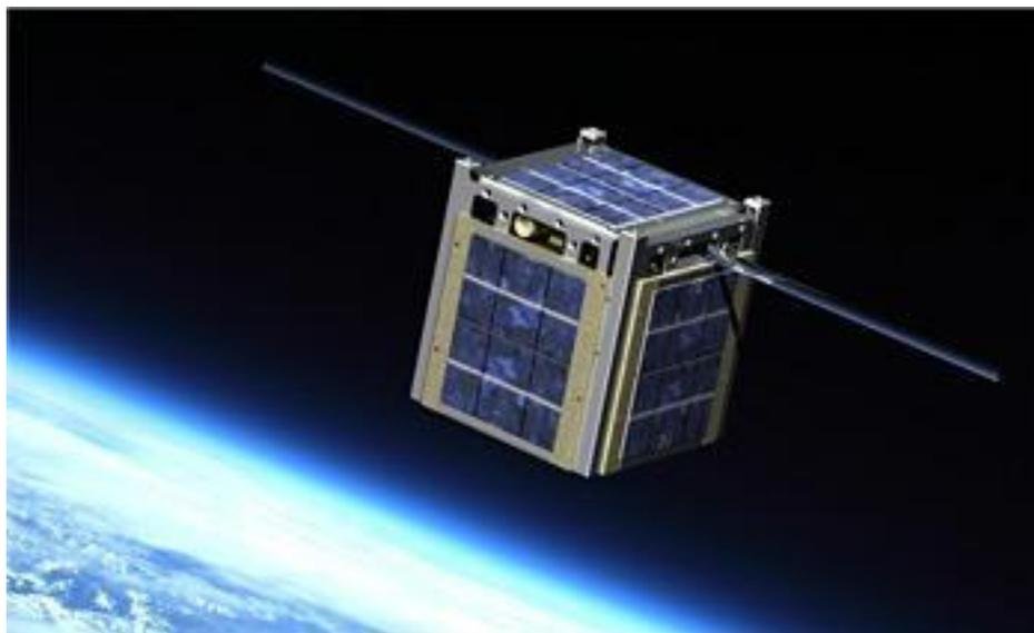
**Figure 1.** An example of a 1U CubeSat [2].
