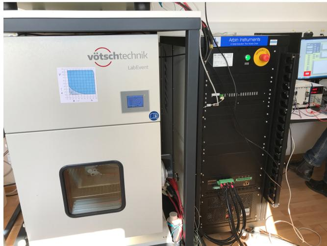
Figure 4.1: Test setup. Left: thermal chamber. Middle: battery tester. Right: test computer.
