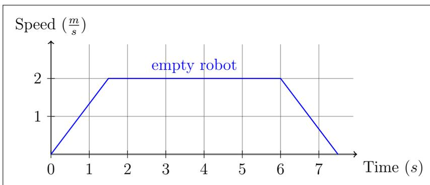
Figure 3: This figure shows the movement of an empty robot in *North* or *South* direction with moving for 2 parking spaces. The total distance traveled is 12 meters, which is exactly the length of 2 parking spaces in that direction.
