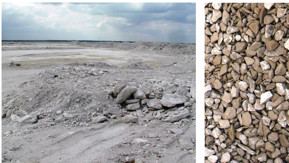
Figure 2. Hydrated oil shale ash: on the ash plateau (on the left) and crushed and sieved hydrated ash (fraction 5–20 mm; on the right).
