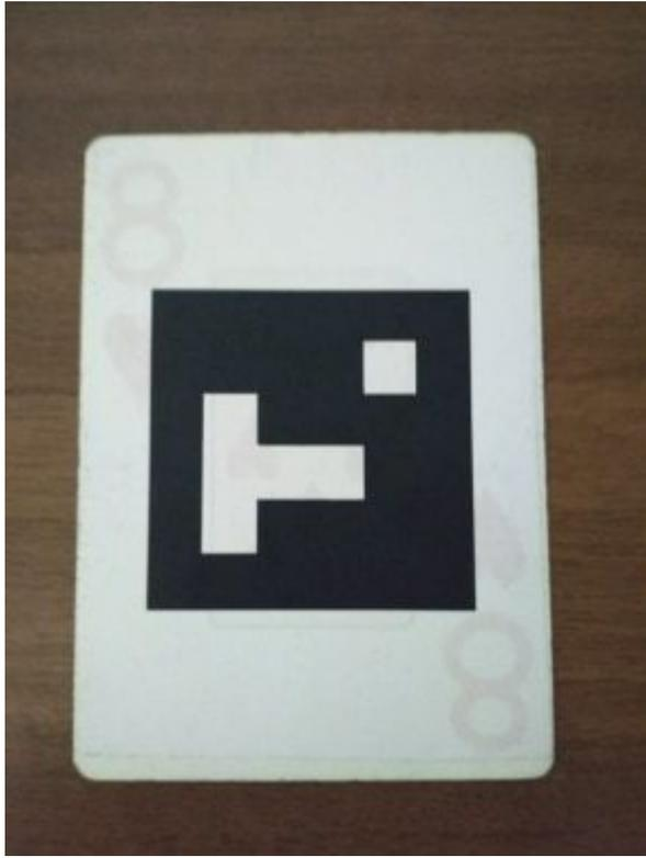
Figure 3.1: Handmade 4x4 dictionary marker
