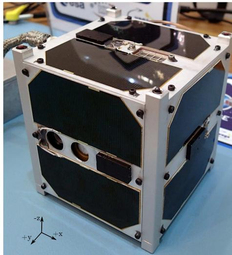
Figure 3.1: ESTCube-1 satellite with axes. Photo: Mihkel Pajusalu.
