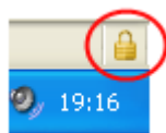
Figure 1.7: A padlock image is created on the status bar every time an https page is being loaded.
