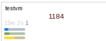
Figure 17. Active VM showing hostname, memory allocated, uptime, processor count and resource usage.
