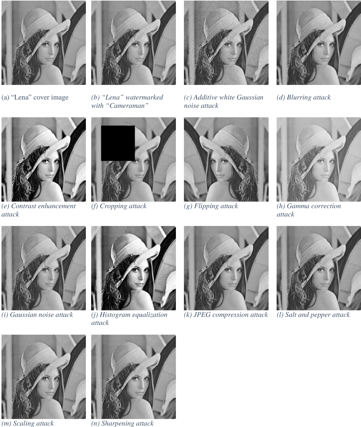
Figure 19. (a) original image, (b) watermarked image, (c-n) watermarked image with different attacks applied to it.
