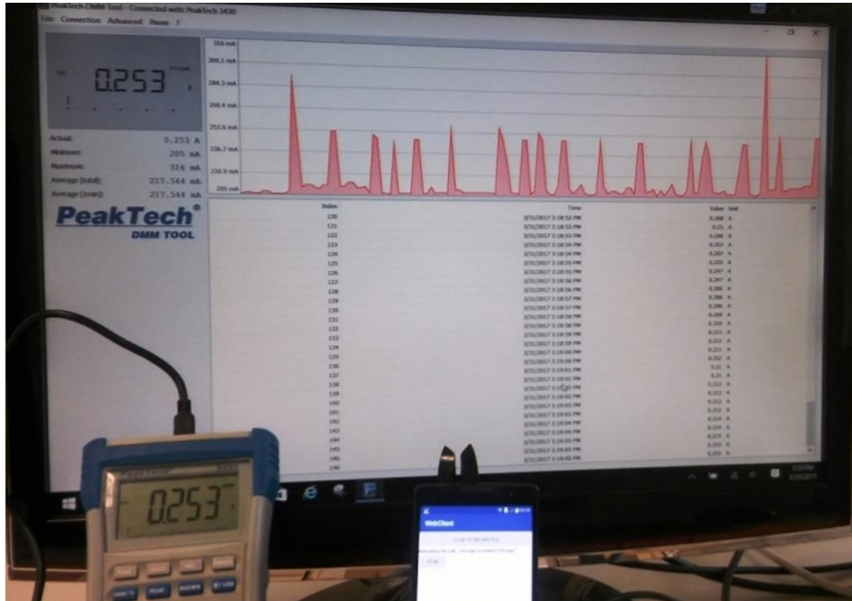
Figure 19: Testbed for the energy measurement
