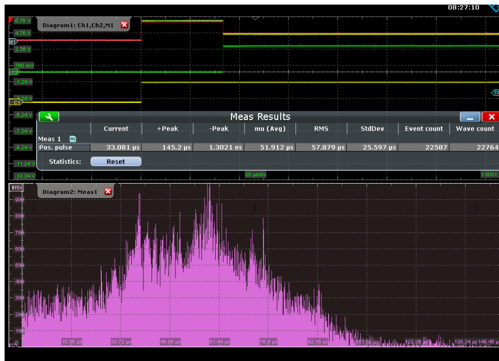
Figure 31: Raspberry Pi 3B and GPS Expansion Board with 4us adjustment and enhanced performance under stress.
