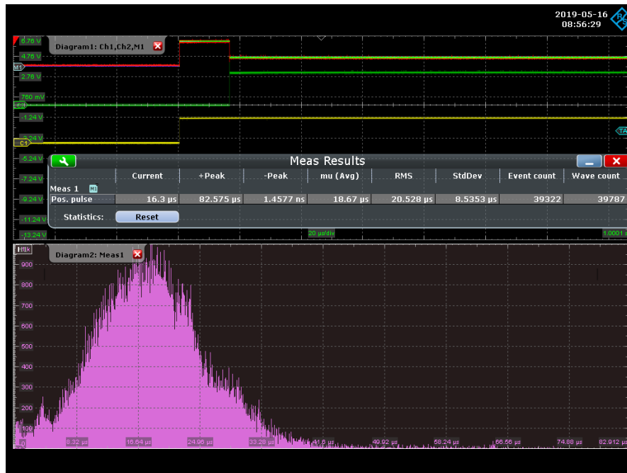
Figure 26: Raspberry Pi 3B and GPS Expansion Board with 4 \mu s adjustment and enhanced performance.
