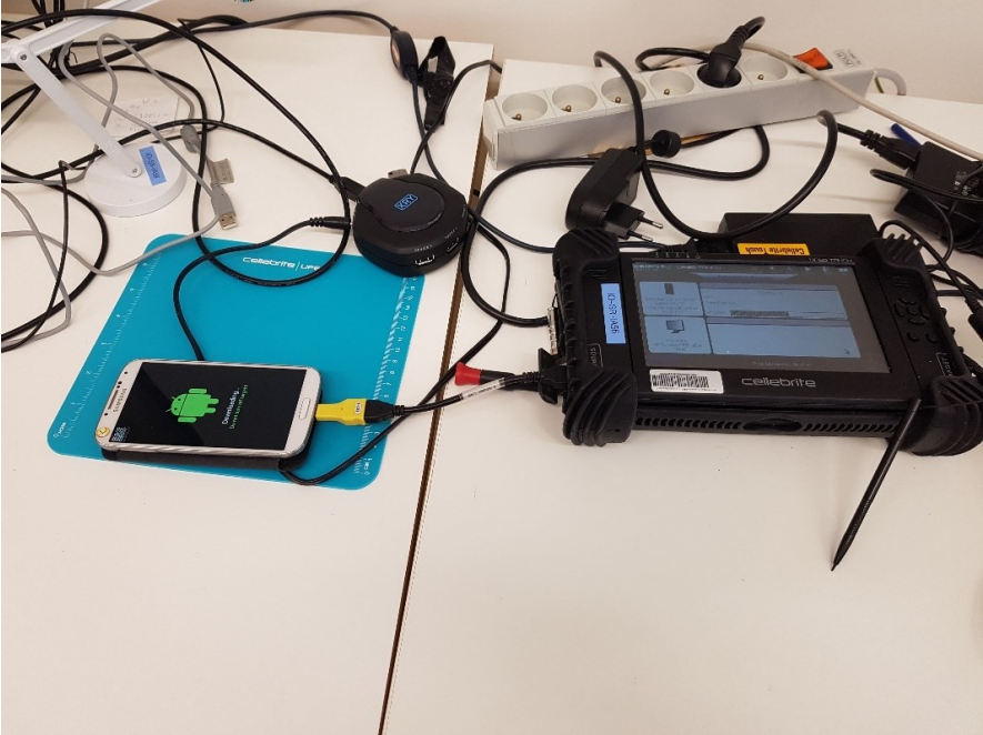
Figure 5 UFED Touch Physical Acquisition Samsung Galaxy S4
