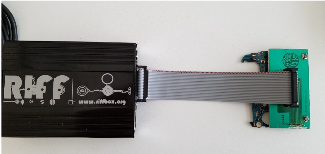
Figure 34 Samsung Galaxy S4 I9505 connected to Riff Box via jig
