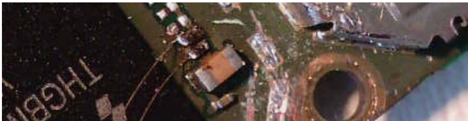
Figure 23 CMD (blue) and CLK (yellod and red) wires soldered close up.
