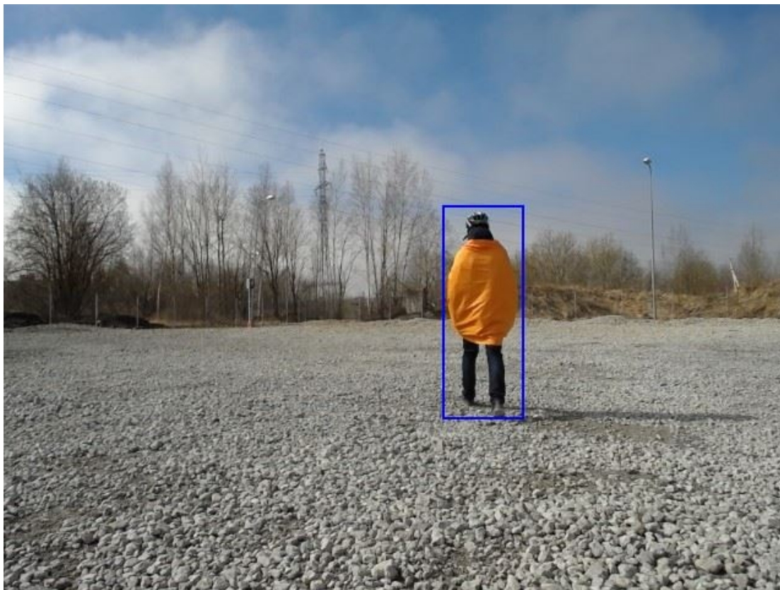
Figure 3. Output of the software based on SqueezeDet's pedestrian tracking. A bounding box is drawn around the person. The approximate angle of the leader on this image is 0.34 radians and the height of the bounding box is 176 pixels.
