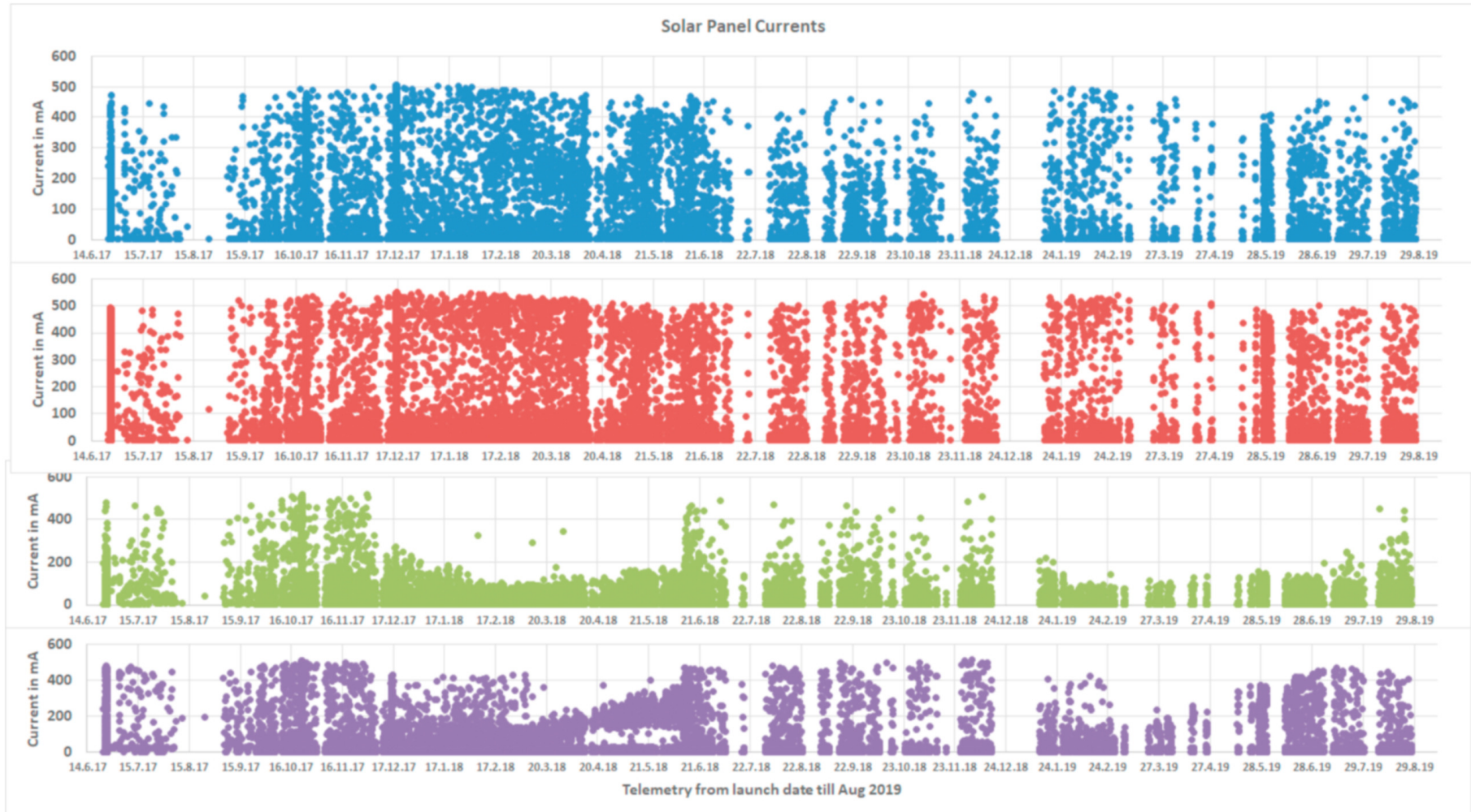
Figure 2.10. Captured intensities of current generated by solar panels starting from launch date until Aug 2019.
