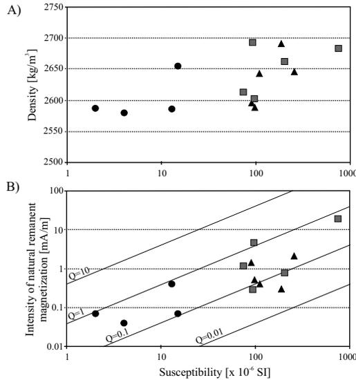
**Fig. 3.** Physical properties of the studied rocks (circle – Silurian, triangle – Ordovician, square – Proterozoic). (A) Density vs. susceptibility, (B) natural remanent magnetization (NRM) vs. susceptibility. Koenigsberger ratio (Q-value) is indicated by inclined lines, the intensity of NRM and magnetic susceptibility are given on a logarithmic scale.
