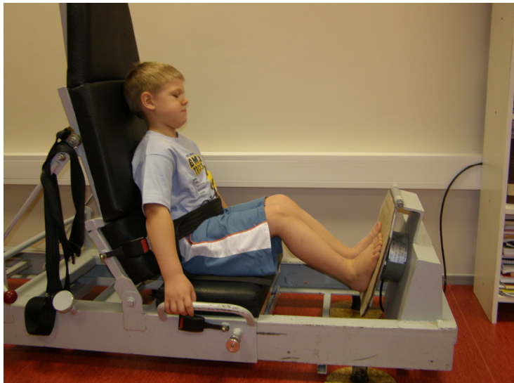
Figure 1. Experimental setup for the measurement of isometric strength characteristics of the leg extensor muscles.
