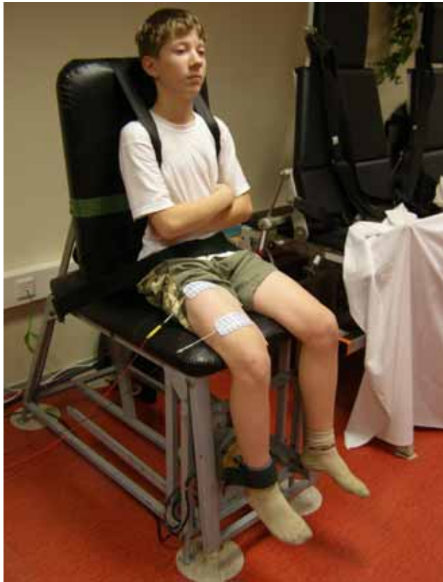
Figure 4. Experimental setup for the measurement of isometric MVC force–time and relaxation-time characteristics, and voluntary activation of the knee extensor muscles.
