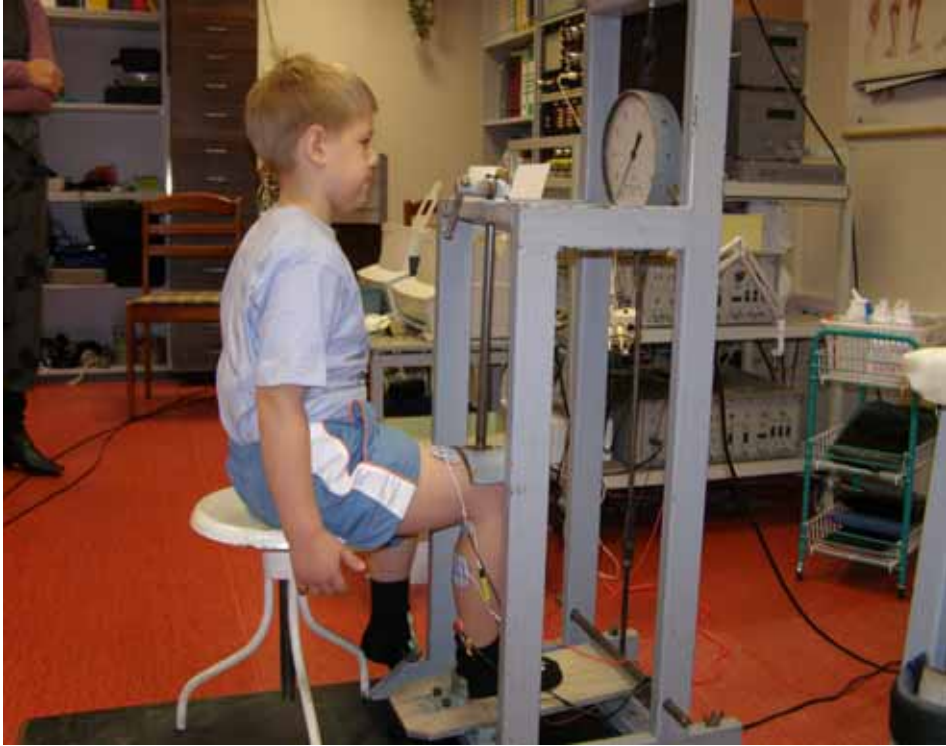
Figure 2. Experimental setup for the measurement of isometric MVC force and electrically evoked twitch contraction characteristics of the plantarflexor muscles.
