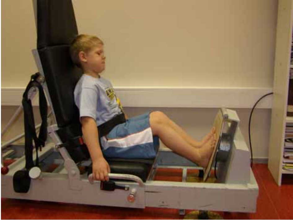
Figure 1. Experimental setup for the measurement of isometric MVC force of the leg extensor muscles.
