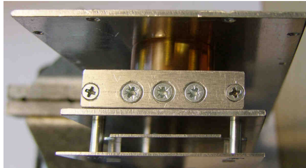
Figure 4.6. Cover of batteries. Be careful to unscrew only two side screws, the other three screws fix the spring contacts and should not be unscrewed.
