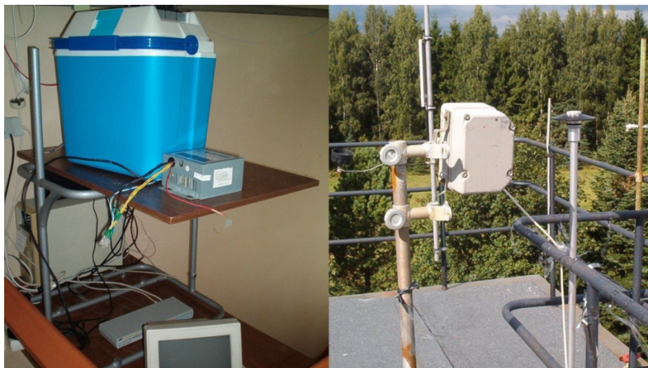
Figure 1. AvaSpec-256 in thermal box (left) and optical head with shutter mechanism at the roof of Tartu Observatory (right).
