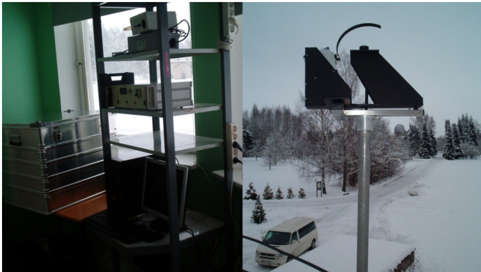
Figure 2. Bentham DMc150F-U inside station (left) and measuring head on the roof of Tõravere meteorological station (right).
