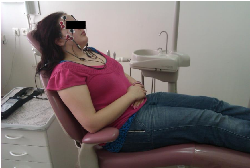
Figure 7. Experimental setup for the measurement of EMG activity. Active electrodes are indicated red and ground electrodes are indicated black.
