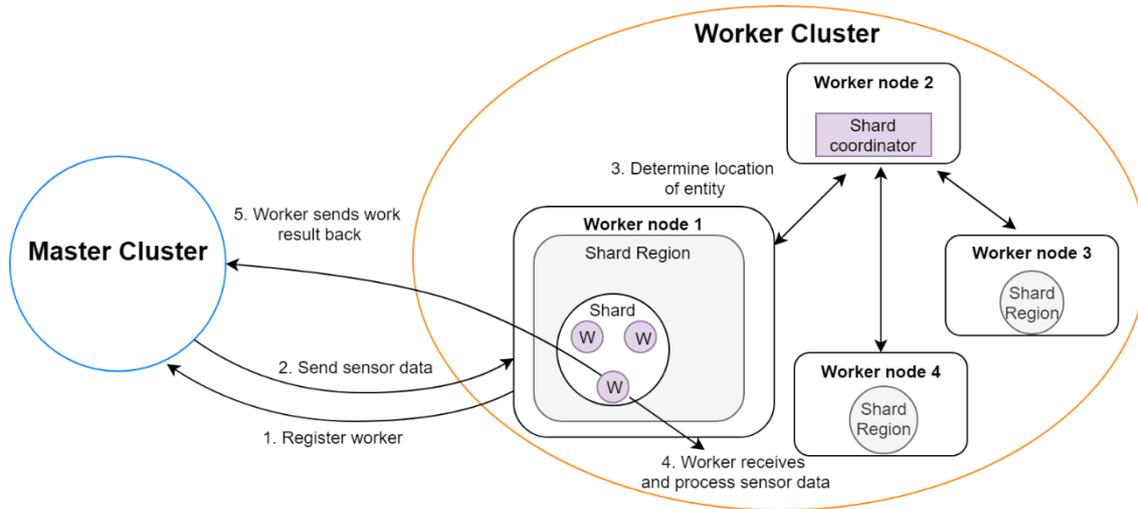
Figure 20. Handling process of sensor data between Master cluster and Worker cluster
