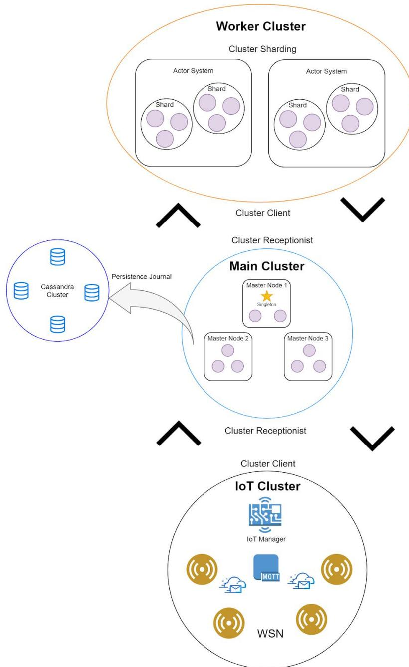
Figure 17. Akka IoT system architecture
