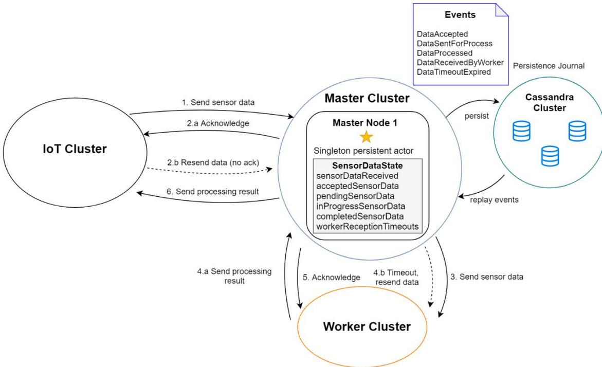
Figure 19. Sensor data handling process by the Master cluster
