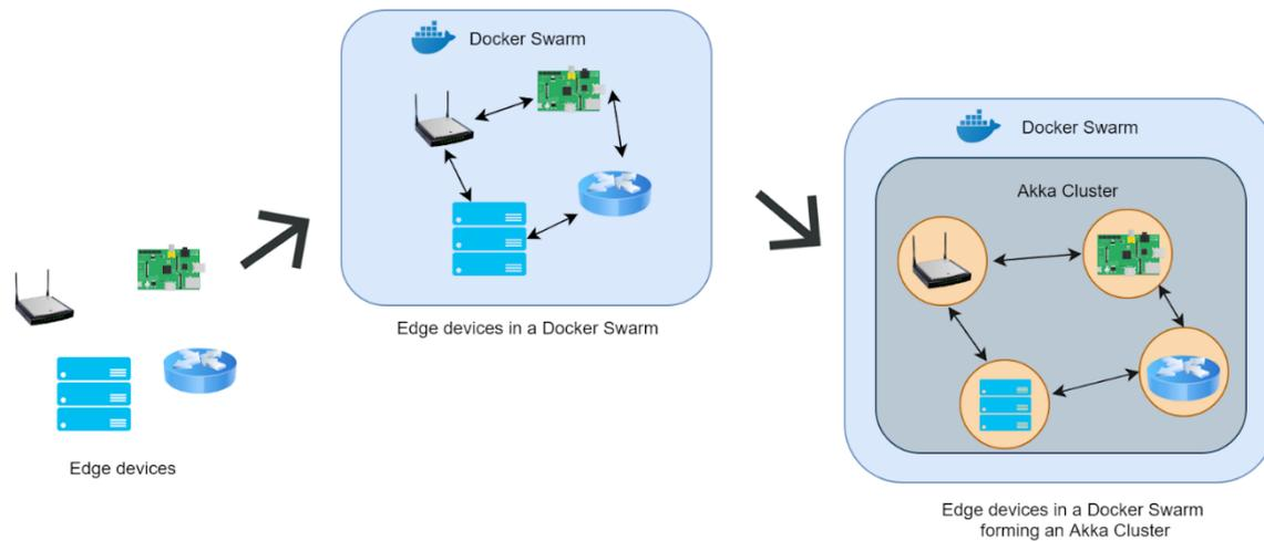
Figure 15. Edge devices forming an Akka Cluster in a Docker Swarm
