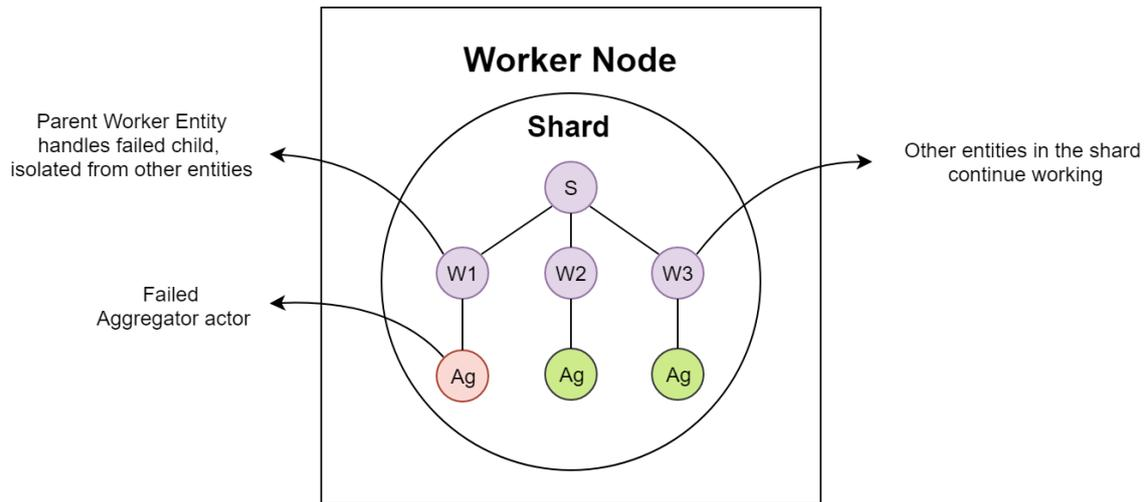
Figure 29. Isolation of failures on a shard
