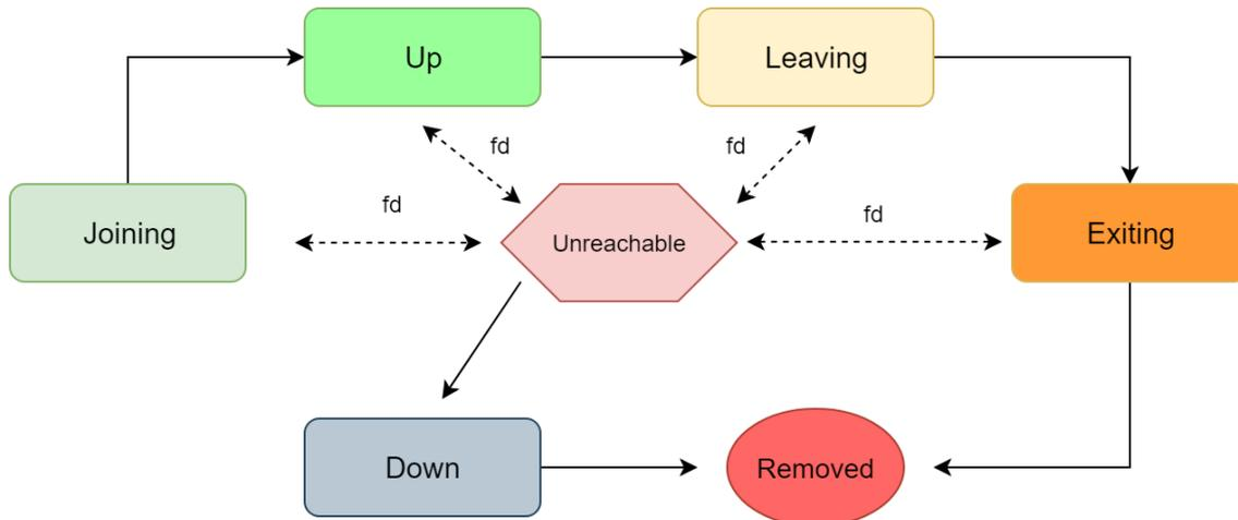
Figure 7. States of a node in an Akka Cluster
