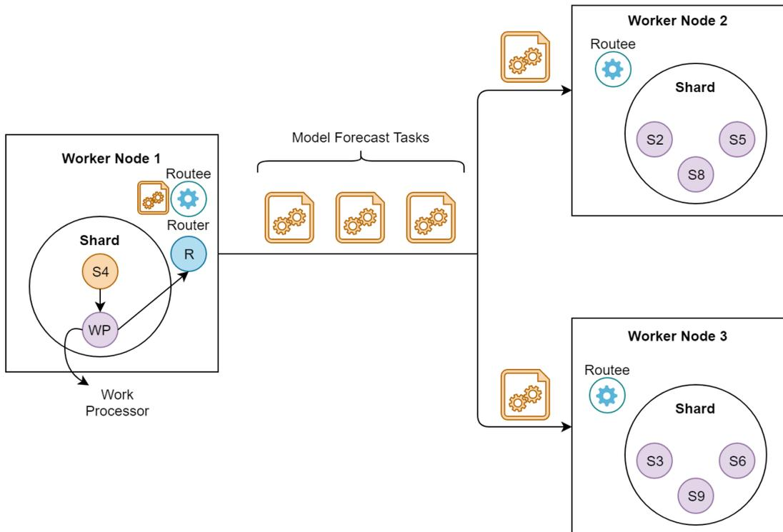
Figure 24. Distribution of computation tasks of a sensor entity in the Worker cluster
