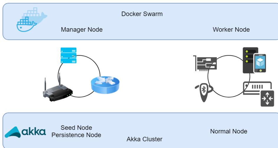
Figure 12. Mapping of Docker Swarm nodes to Akka Cluster nodes
