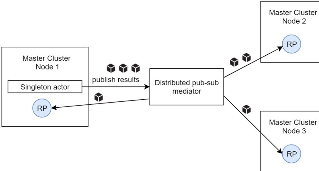
Figure 25. Distribution of results using Distributed pub-sub mechanism
