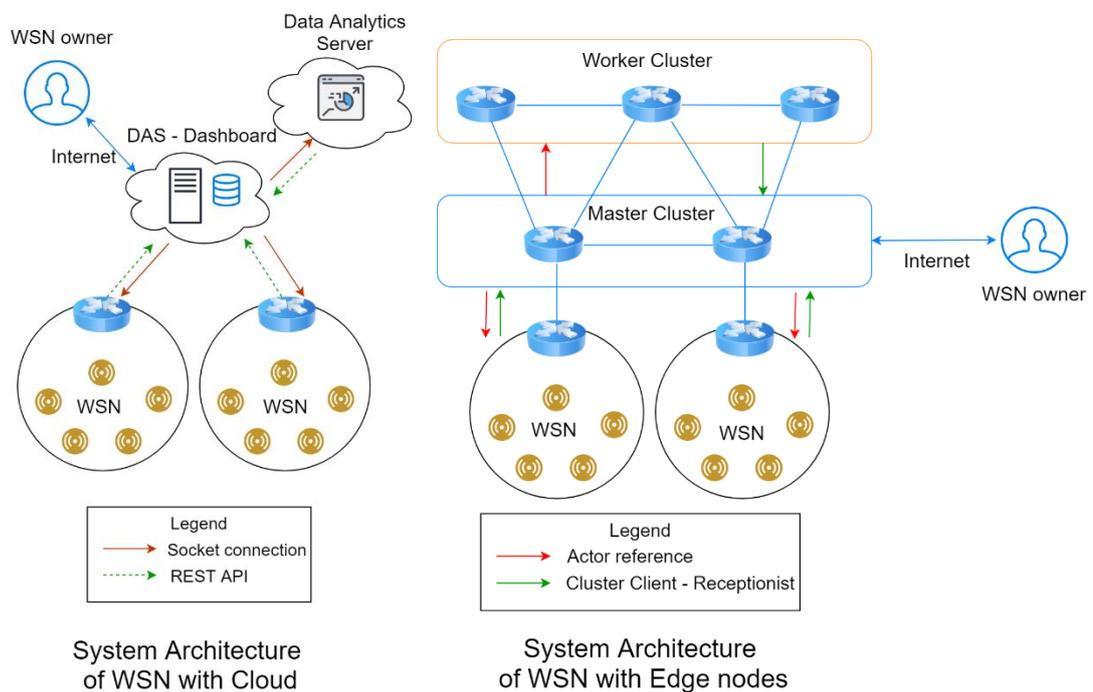
Figure 16. Cloud and edge IoT architectures
