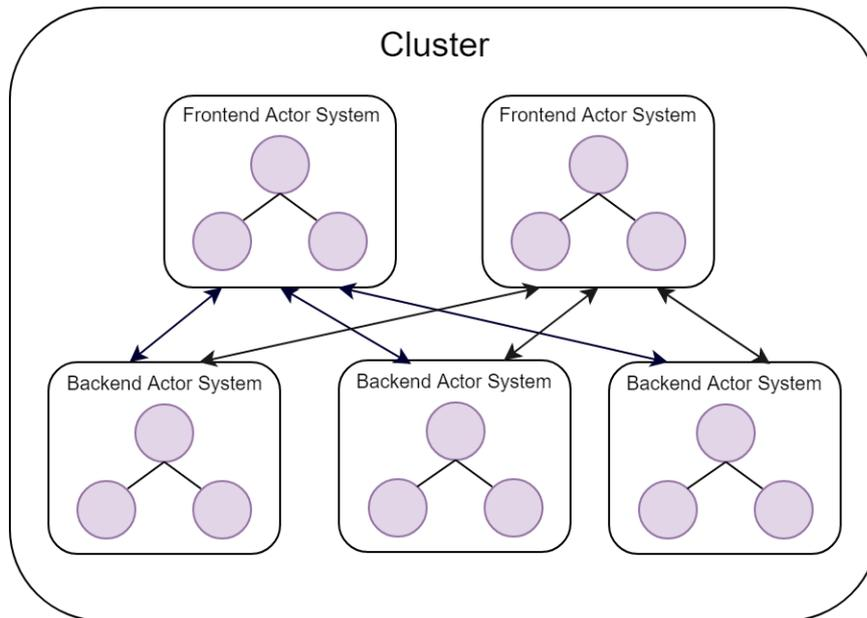
Figure 13. Cluster using Frontend and Backend actors
