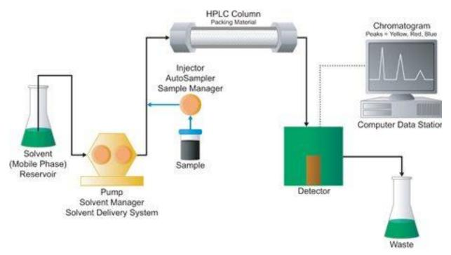
Figure 2-1 High-Performance Liquid Chromatography (HPLC) System
