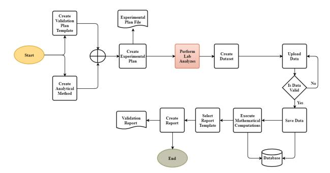
Figure 3-2 Flowchart of the validation process using ValChrom
