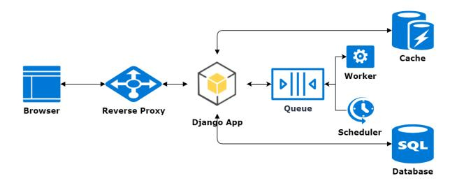
Figure 3-1 System Overall Architecture
