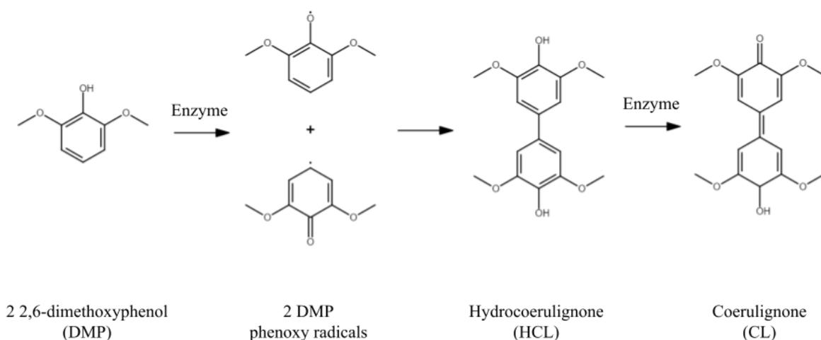
**Figure 10.** DMP conversion to CL: enzyme catalyzes the oxidation of DMP to the corresponding phenoxy radical; phenoxy radicals non-enzymatically dimerize to hydrocoerulignone (HCL); enzyme catalyzes the conversion of HCL to chromogenic CL (Marvin JS, Google Slides).
