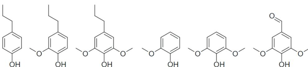
**Figure 4.** (from left to right) Phenolic substrates of laccases originate from lignin phenolic units, differentiated by the number of methoxy substituents: p-hydroxyphenylpropane, guaiacylpropane, syringylpropane. The most commonly used laccase phenolic substrates are guaiacol, 2,6-dimethoxyphenol, syringaldehyde (Marvin JS).
