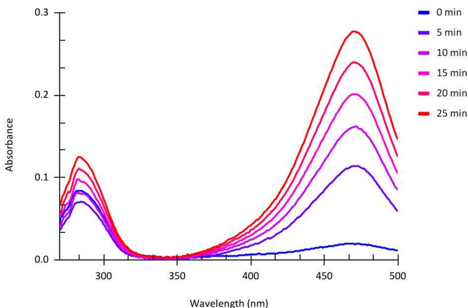
**Figure 17.** SVLAC spectral assay with DMP was carried out using 2 mM DMP and 10 nM SVLAC. SVLAC spectral assay of DMP conversion to CL did not detect side products. The increase of CL absorbance at 469 nm wavelength and the changes of HCL and DMP absorbance at 280 nm wavelength are in agreement with the three-step model of DMP conversion to CL.
