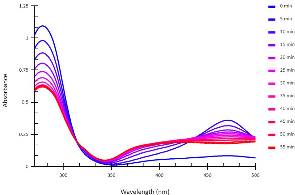
**Figure 18.** SVLAC spectral assay with HCL was carried out using 60  $\mu\text{M}$  HCL and 5 nM SVLAC. SVLAC spectral assay of HCL conversion to CL detected at least one side product, which absorbed approximately between 350 to 430 nm wavelengths. The decrease of CL absorption at 469 nm deviates from the three-step model of DMP conversion to CL.
