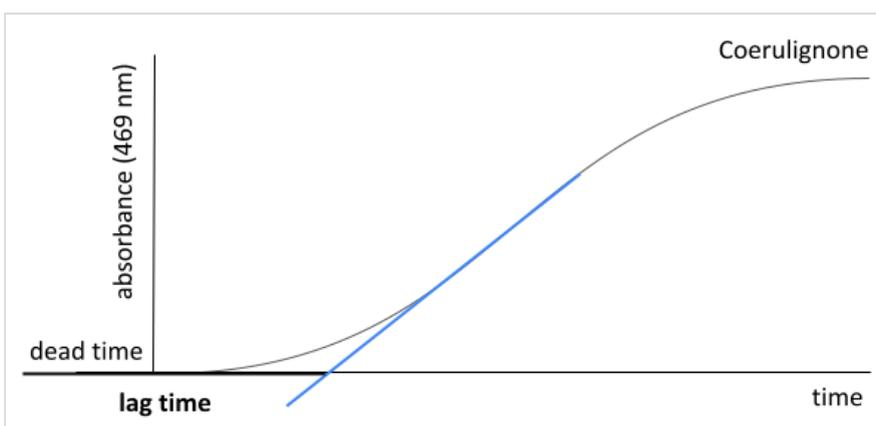
**Figure 15.** SVLAC lag time determination: the CL formation curve was extrapolated and the intersection point of this line and x-axis was defined as the starting point of CL formation. The time period from initiation of the reaction to the starting point of CL formation was defined as the lag time.
