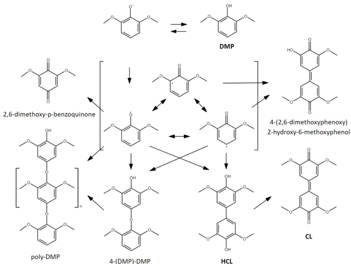
**Figure 12.** Possible oxidation products of DMP: monomeric 2,6-dimethoxy-p-benzoquinone by oxidation and oligomers through two oxidative couplings: 4-(2,6-dimethoxyphenoxy)-2,6-dimethoxyphenol is formed by C-O dimerization and can be further polymerized; HCL is formed by C-C dimerization and can be further converted to CL; 4-(2,6-dimethoxyphenoxy)-2-hydroxy-6-methoxyphenol is formed by intermediate oxidation to 2-hydroxy-6-methoxyphenol and subsequent C-O coupling (Marvin JS, Google Slides).
