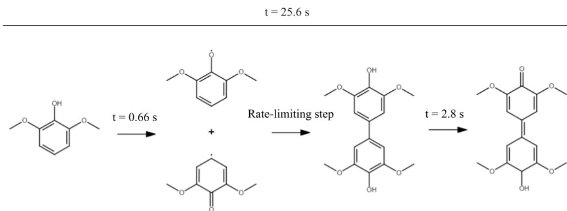
**Figure 19** Rate-limiting step of SVLAC-catalyzed DMP conversion to CL: the whole conversion of DMP to CL takes about 25.6 s. It starts with the first enzymatic step with the lowest transit time of 0.66 s. Then it is followed by a rate-limiting step, the non-enzymatic conversion of DMP radicals to HCL. Finally, the second enzymatic step takes place with moderate transit time of 2.8 s (Marvin JS, Google Slides).
