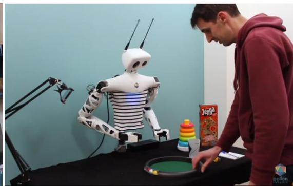
**Figure 2.** *Tele-operated robot “Reachy” by Pollen Robotics. This robot can be operated through VR. In the example pictures above a game of dice is played through it [18].*
