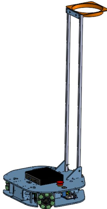
*Figure 6: Modified Robotont platform for the Roboquiz game. Drawing done in SolidWorks*
