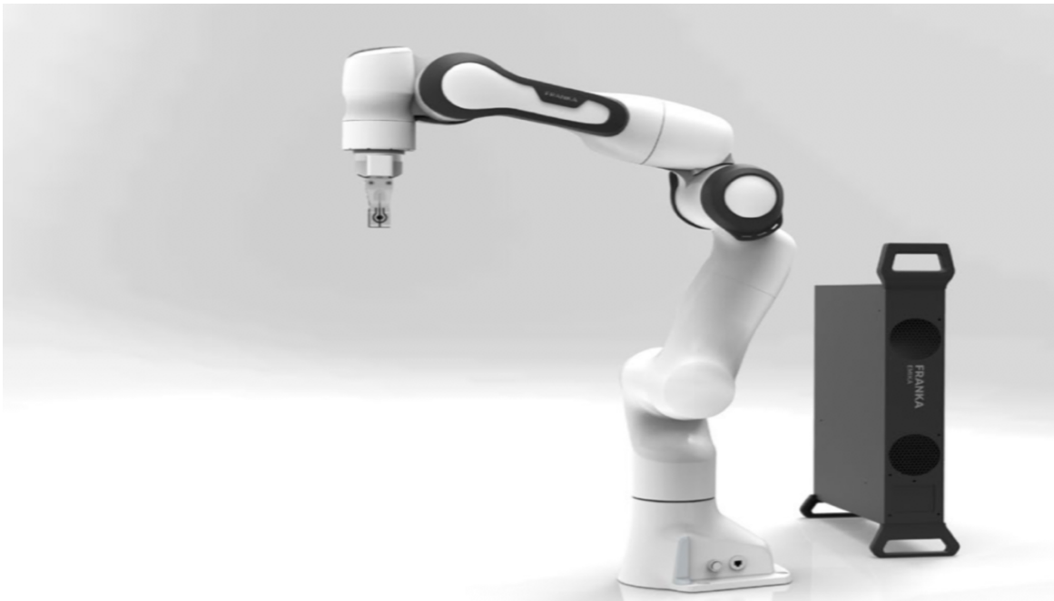
Figure 4.5: Franka Emika Panda manipulator and its controller [30].
