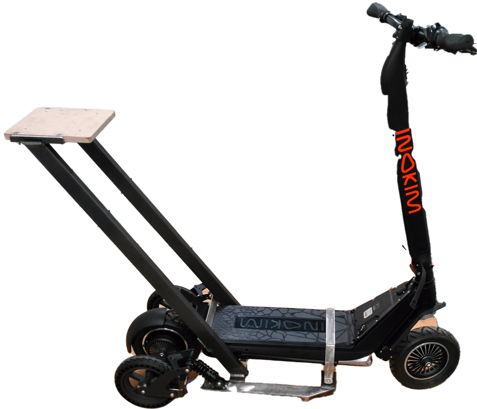
Figure 2. The platform equipment rig, where sensors, damping system, and the compute board are mounted.
