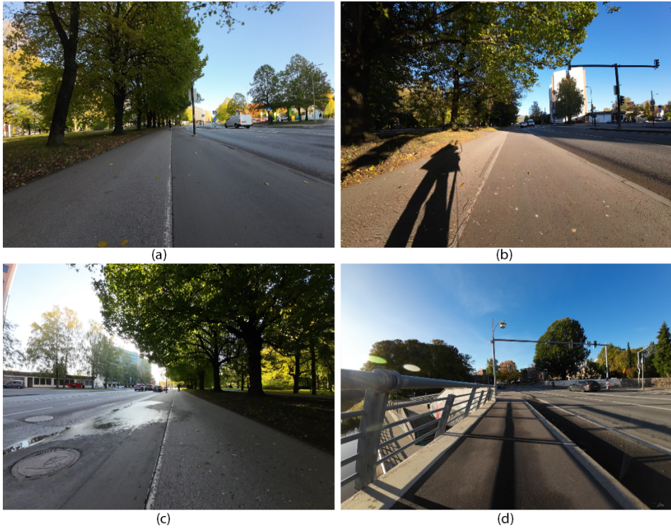
Figure 33. Analysis of the system failure scenarios: (a) lack of distinguishable landmarks in the scene, (b) landmarks concealed by vegetation such as trees, (c) obstruction caused by urban structures or elements, (d) diminished visibility due to sun glare and constraints arising from inadequate model training.
