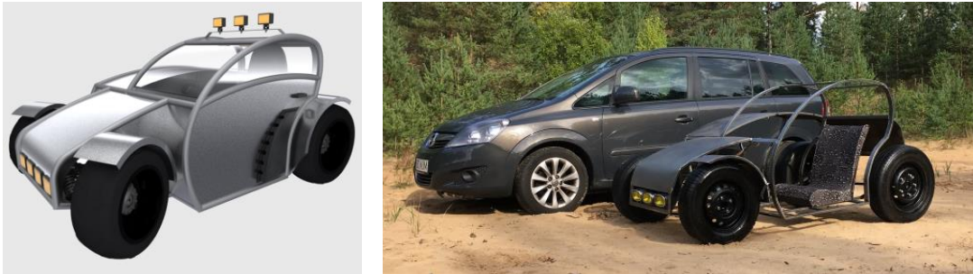
Figure 5. 3D model of didactic vehicle and comparison of vehicle frame with passenger car
