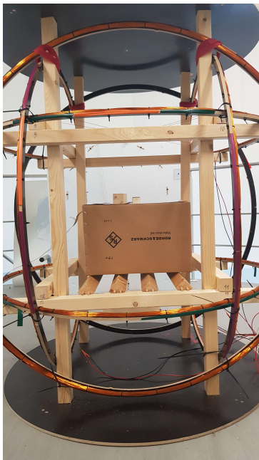
Figure 8. Helmholtz coils with magnetometer on a cardboard box
