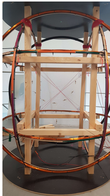
Figure 9. Helmholtz coils with twisted polyamide cord for finding the center
