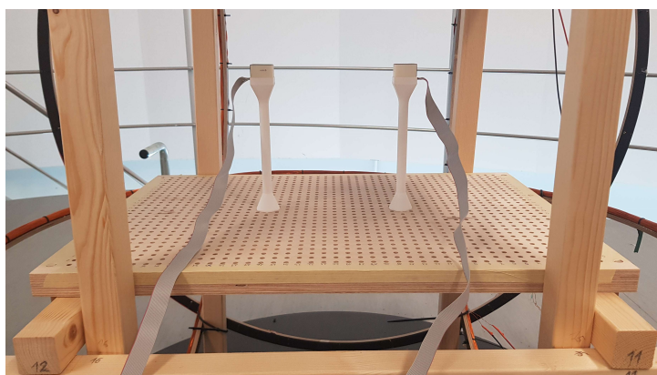
Figure 11. Magnetometers connected in test configuration to the underboard using magnetometer holders
