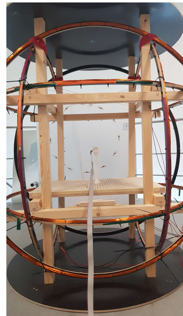
Figure 10. Helmholtz coils with underplate and magnetometer in the center
