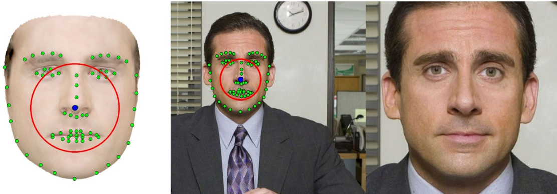
Figure 11. Centre points (blue points), average distances from the center point (red circles), and the corresponding crop result. Left: rendered model. Centre: input image. Right: cropped result.
