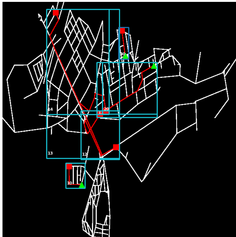
Figure 8. A ground truth image of the optimal snowplow routes with the training bounding boxes plotted.
