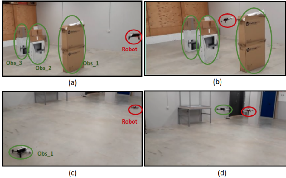
Figure 20. Snapshots of real-world experiments utilizing our optimizer in both a static (a-b) and dynamic (c-d) environment. Obstacles are marked in green, and the robot is shown in red. In (c-d), the dynamic obstacle is represented by a moving robot.
