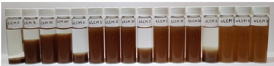
Figure 15. Solution stability of LCM, eLCM, tLCM and nLCM with varied US treatment from 0–20 min at 0.3% cellulose content, which means varied total loading due to e-, t-, nLCM having less lignin in the mix and thus more cellulose. The stability of water dispersion after 72 h of storage is shown.
