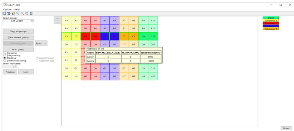
Figure 3. Graphical user interfaces of Export Tools module with IQMTools/ SBToolbox2 export preview and the grouping of a receptor concentration determination FA experiment. Export Tools main interface (A) allows to choose the number of groups and their names in the “Group wells” panel, enter calculation formulae in the “Formula panel”, make adjustments to the experiment time-line in the “Remove timepoints and change units” panel and adjust SB software specific parameters in the “Export preview” panel (A). The grouping view of the Plate Simulator (B) allows to group and subgroup wells, set blank wells or set specific time-points or sets of time-points of wells as timewise blanks. Wells have specific color-based highlighting and tooltips based on the grouping, treatment and events to allow quick and accurate overview of the experiment and current grouping settings.
