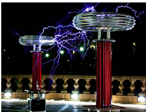
Joonis 5.1: Zeusaphone - muusikaline Tesla Trafo. Pilt pärit internetist, autor: Iosif Aragiannis, veebileht: https://mct-master.github.io/interactive-music/2022/11/26/iosifaragiannis-zeusaphone.html
