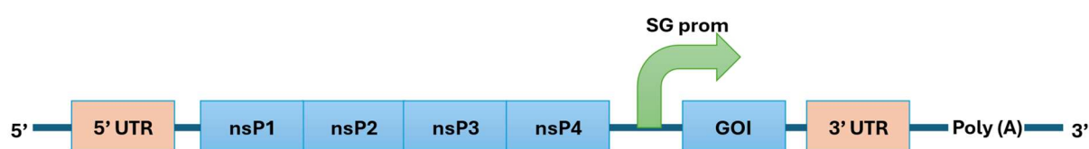
Figure 4. Schematic structure of an alphavirus replicon carrying a gene of interest. The replicon contains the 5' untranslated region (5' UTR), the nonstructural protein coding region nsP1–nsP4, a subgenomic promoter (SG prom) driving expression of the inserted gene of interest (GOI), followed by the 3' untranslated region (3' UTR) and poly(A) tail. The structural genes are replaced by the GOI, allowing RNA replication and reporter/transgene expression without production of infectious virus particles in the absence of helper structural proteins.
