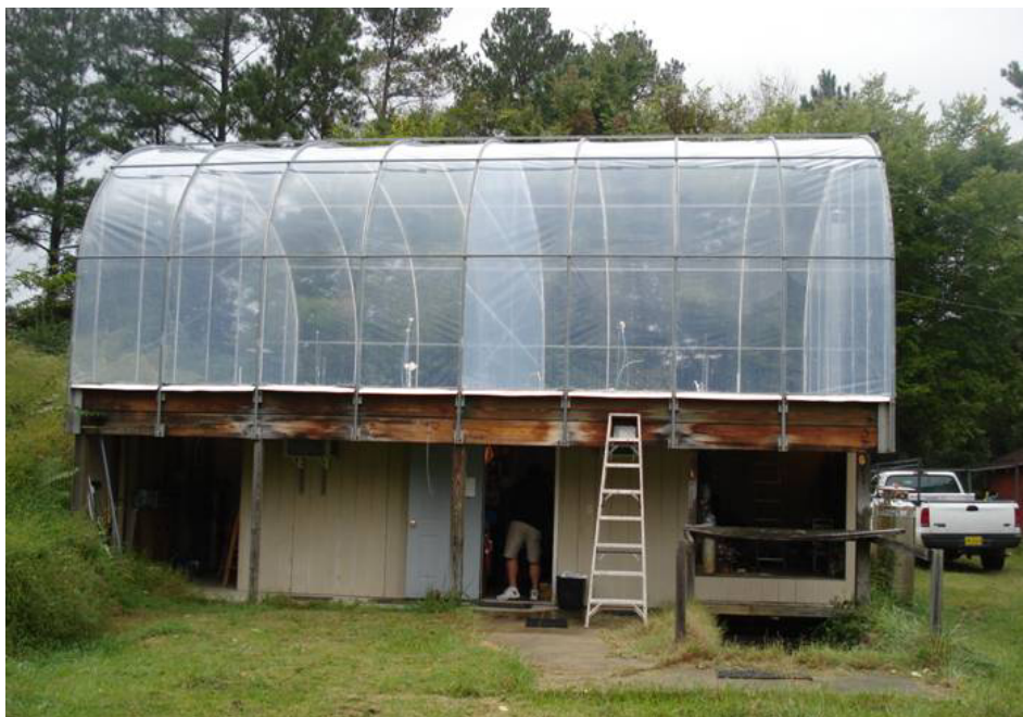
Figure 2. The dual outdoor Teflon Film smog chamber of UNC at Chapel Hill (NC, USA)
