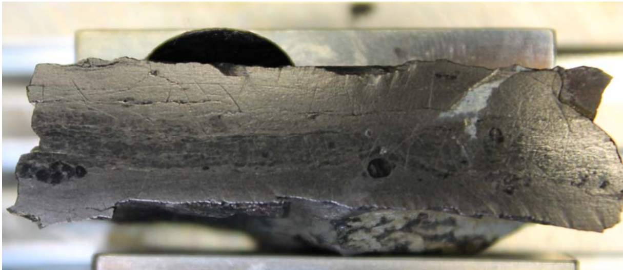
Figure 4: A polished surface of a sample from Shunga village outcrop organic-rich mudstone. Abundant dark phosphatic layers and nodules are visible. The length of the sample is approximately 4 cm.
