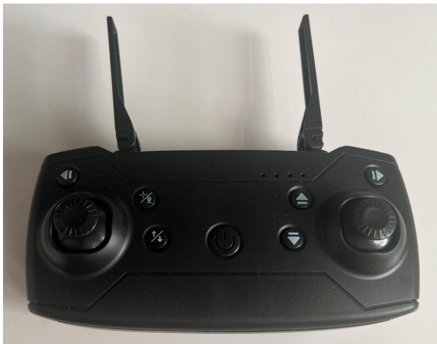
Figure 5 Remote control for the drone with phone holder retracted and fake antennas
