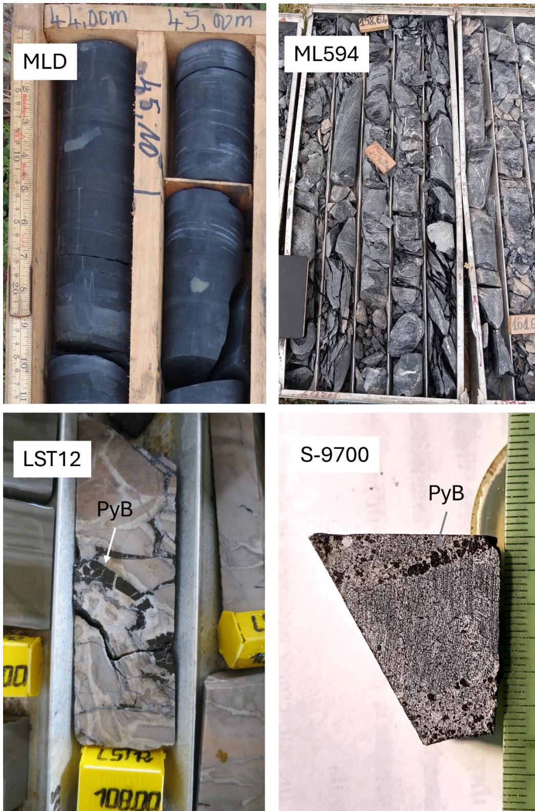
Figure 6. Different host rock for samples. Black shales of MLD and ML594 drillcores, brecciated dolostone from LST12 and conglomeratic sandstone in Sully drillcore, sample S-9700.
