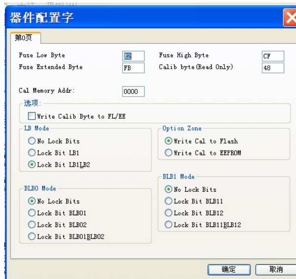
Figure 4.2: The screenshot we received that shows the fuse values of the microcontroller taken from the car module
