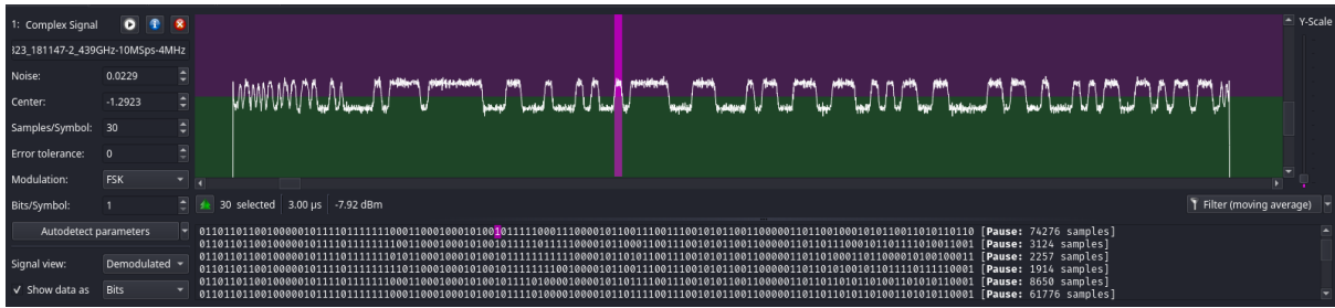
Figure 100. Demodulated Hama mouse's packet
