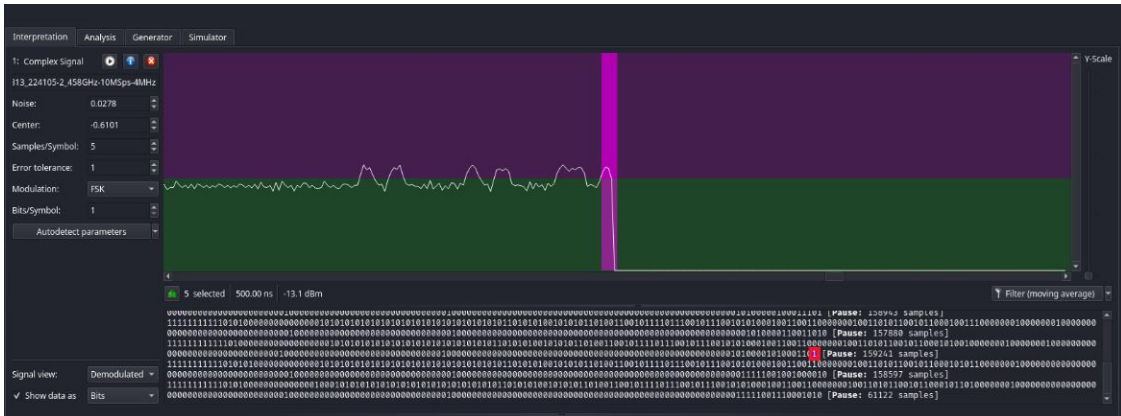
Figure 28. Visualization of the last wave of a packet being interpreted as binary 1
