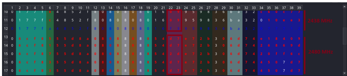
Figure 99. Comparison between “7” key press and “key release” Hama keyboard’s packets in two different frequencies
