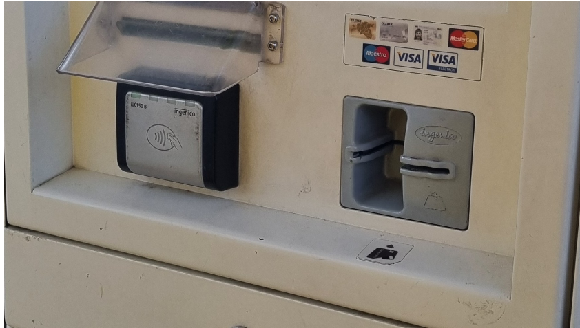
Figure 3. Ingenico iUC150B and iUR250 terminals found in Olerex gas station.
