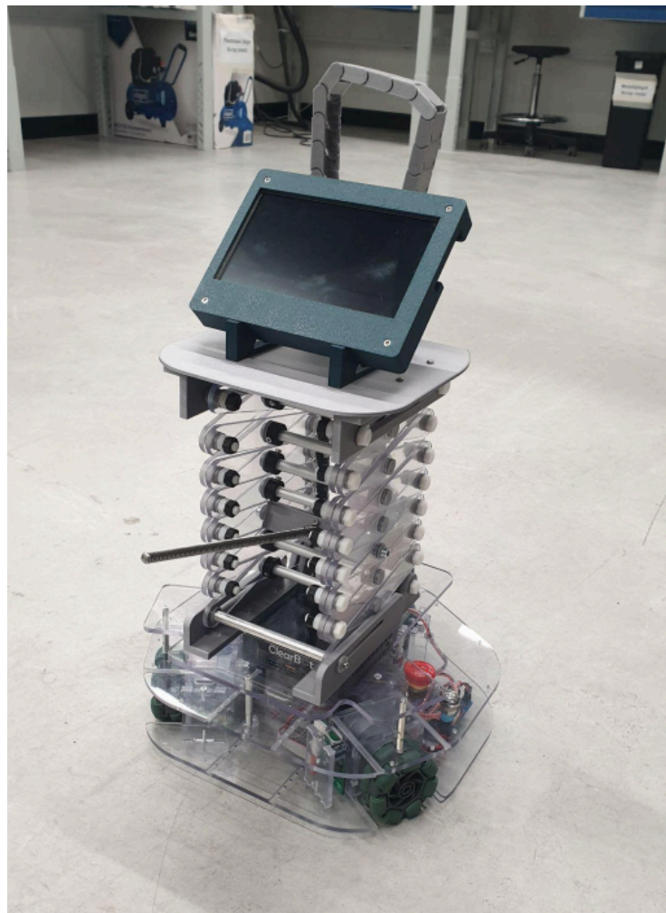
Fig. 2. Height adjustment mechanism platform for Robotont.
