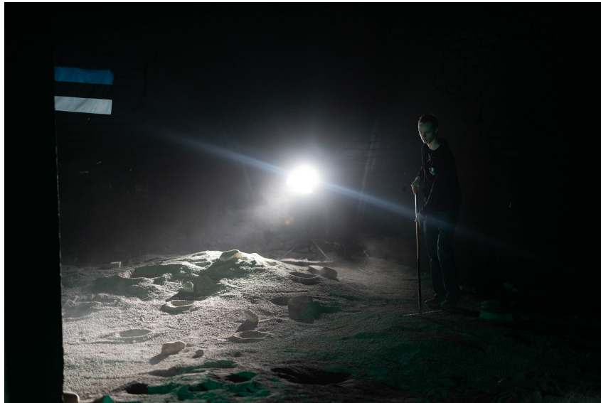
Figure 3.3: The lunar analogue site is being readied for a KuupKulgur test. Notice the prepared ground features (rocks and craters) and the searchlight providing a sunlight analogue.
