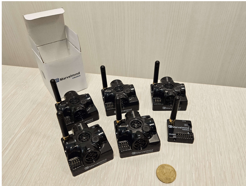
Figure 3.4: The starter set of beacons by Marvelmind used for testing.
