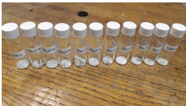
Figure 8: A series of Zn_xCd_{1-x}WO_4 crystals used in measurements.
