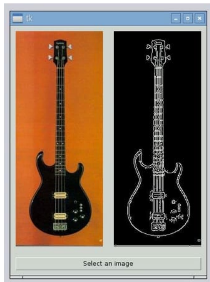
Figure 1: Loading an image, computing edges using the Canny edge detector, and then displaying the result using Tkinter and OpenCV.
