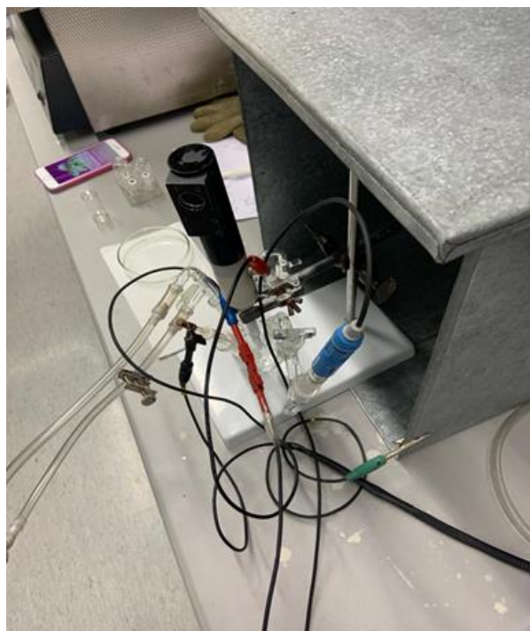
Figure 6. Picture of the 3-electrode system used for electrochemistry measurements.
